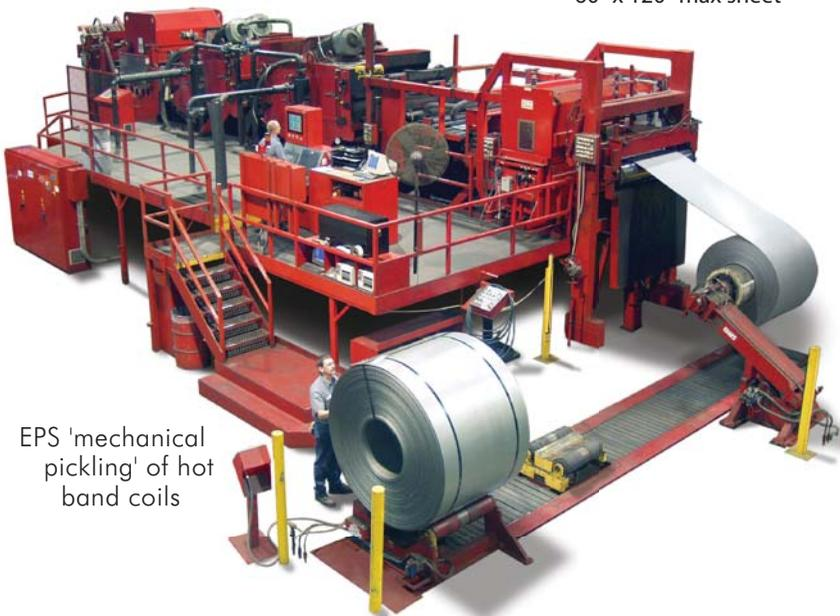
EPS 'mechanical pickling' of hot band coils
